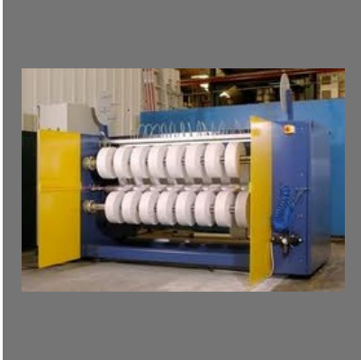
Slitting Facility for Textile
